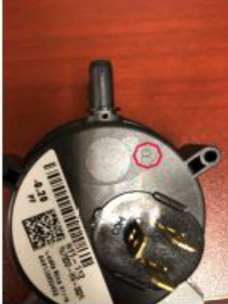
Pressure switch side "P"
