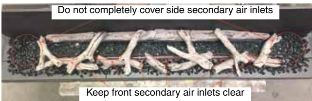
Correct Black Coal placement
