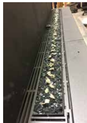
Burner covered with Fireglass and glowing wool
